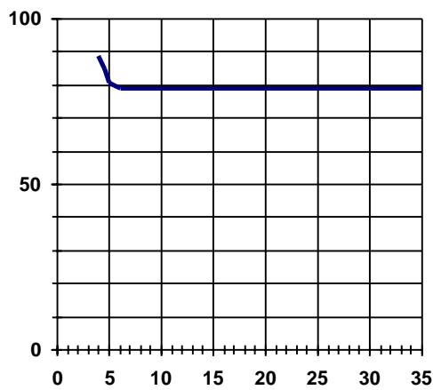
Figure 7 - R ds(on) (mΩ) Vs V CC (V)
