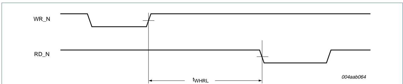
Fig 17. ISP1582 ready signal timing
