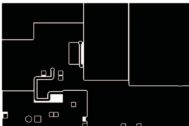
Figure 45. TPS40200EVM-001 Bottom Copper (X-Ray View from Top)
