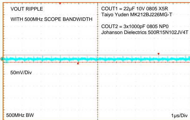
Figure 75. 500 MHz Oscilloscope Bandwidth, 3x1000 pF additional output capacitance Output Voltage Ripple and HF Noise V_{OUT} = 5.0\text{ V}
