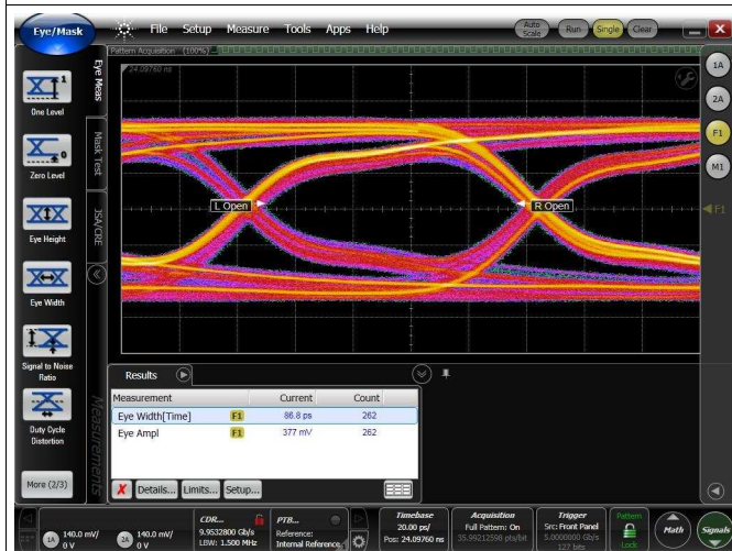
Figure 9. 5 Gbps Source Eye Diagram
